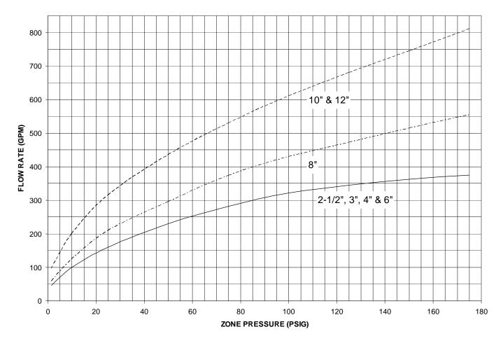
Relief Valve Discharge Rates Model RP4A & RP4AN
